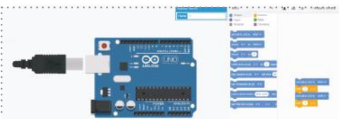
Use Blockly or Scratch to code an Arduino microcontroller. Sample Project (Blinking board led (Pin 13) with block coding)
